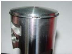
Install the ring on the piston so the ends are aligned with the retaining pin as shown.
