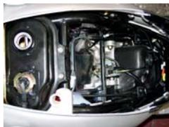
Remove the spark plug cap. Remove the rear fan cover screw near the intake manifold. Disconnect the oil pump cable.
