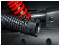
Squeeze the clamp with 2 fingers and remove the air inlet pipe from the air box.
