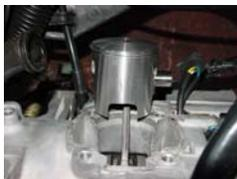
Make sure the base gasket surface is clean and with a clean towel in the crankcase install the piston on the rod. Install the other circlip exactly the same way as the one before.
