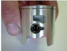
Make sure the circlip is in the exact position shown so there is no chance of the clip coming out at high rpm.
