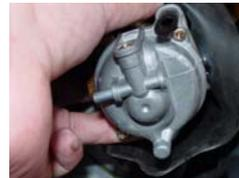
Remove the float bowl being very careful not to bend the float level adjustment! Note the location of the main and low speed jets. The main is in the center. They are about to get larger!
