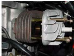
Completely unscrew the (4) 7mm cylinder studs and remove the studs, cylinder head and head gasket.
