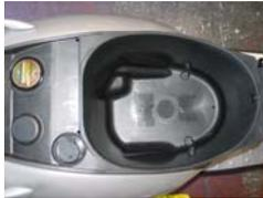
Open seat and remove the (2) rear luggage box bolts. The (2) cap nuts at the bottom of the box. There is also a large Philips screw underneath the seat hinge. Remove the oil cap and rubber washer. underneath.
