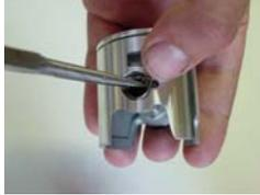
Push the new wrist pin into the bosses just shy of the groove for installing the circlip. Then install the left hand circlip first. Then remove the wrist pin. Note the arrow on the top of the piston faces towards the exhaust.
