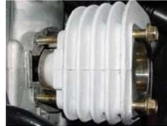
Remove the 2 studs and slide them through the cylinder head and head gasket using the same as above procedure. Torque all four studs to 1.4-1.7 kg. Tighten slowly and evenly in an X pattern. Install the air shroud. **For Cobra Airsal cylinders add (2) 7mm washers to each stud to compensate for the different cylinder/head dimensions.**
