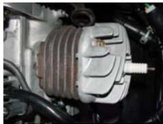
Loosen the (4) cylinder studs and lightly tap the cylinder to loosen the base gasket.
