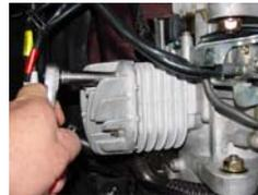
Install the oil pump cable. Make sure the lock nut is secure!
