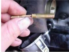
Unscrew the low speed jet and drill out with the neat jet drill I got here.
