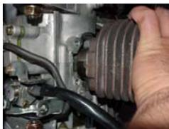
Remove the cylinder carefully avoiding any material from falling into the crankcase.
