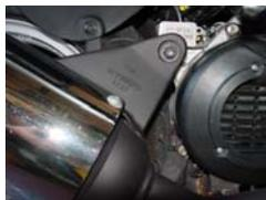
Remove the (1) 8mm exhaust bolt and loosen the other. Remove the 6mm fender bolt.
